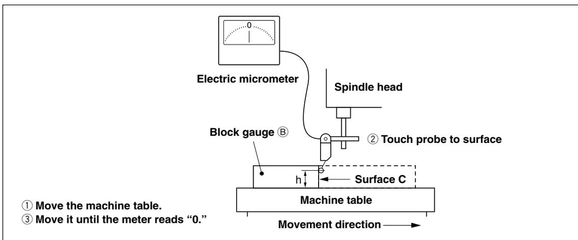
Note: Do not change the probe height h until finished measuring.
